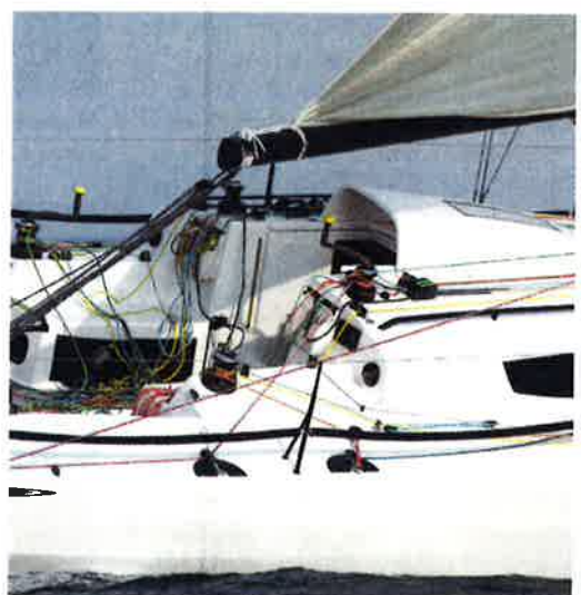
Primary winches are easy to get to without facing leeward and outboard, and there is plenty to brace yourself against when working the secondary winches
