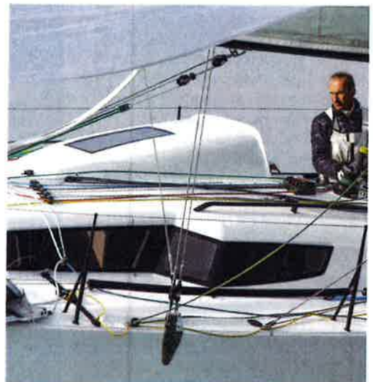
The coachroof 'bubble' module provides protection for the companionway area as well as facilitating a good view of the rig and sail plan from below
