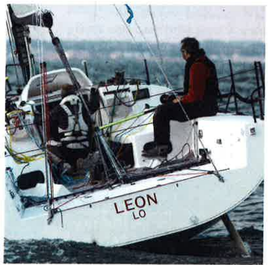
The yacht has twin rudders, but a single tiller, which provides more space in the cockpit than twin tillers. A single rudder can be fitted for inshore racing
