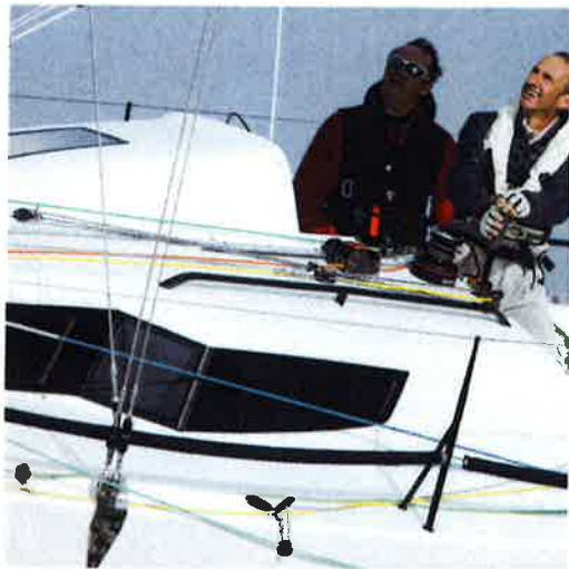
The stepped coachroof windows are much more than a styling detail; they allow more space for the transverse jib car tracks and assist forward visibility from below
